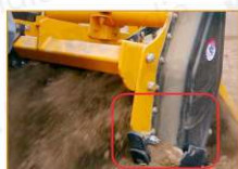
Skid Cover • Improves strength and durability of skid shoes • Less maintenance cost
